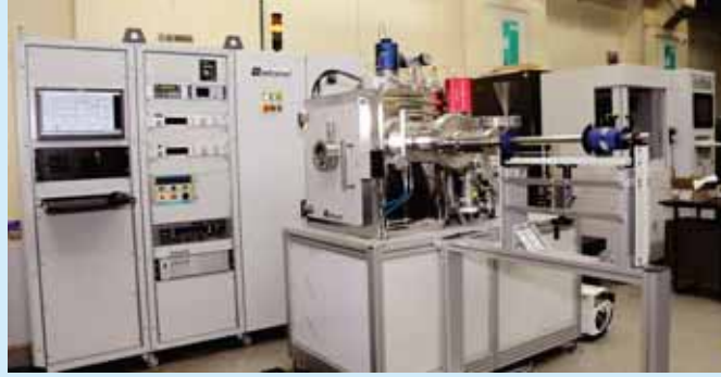
Plasma Vapour Deposition (PVD) Facility at CMTI
