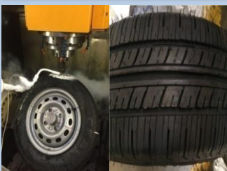
Machining of Tyre Treads - Cryogenic Machining
