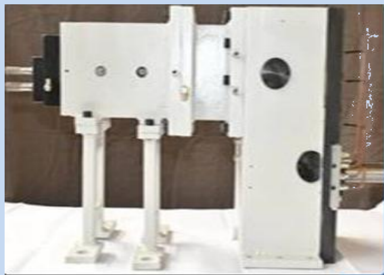
Twin Screw Gearbox
