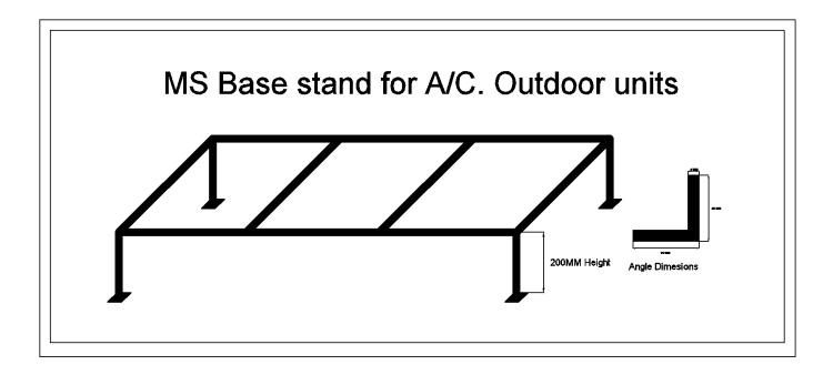
Note: Fabrication as per drawing attached with L angle bar size of 40mmx40mmx5mm
