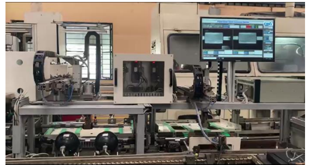
Fluted Roller Vision Inspection System
