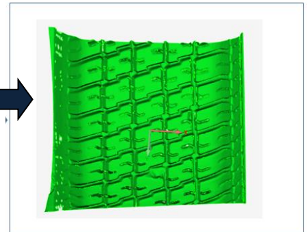
3D Point Cloud generation and registration
