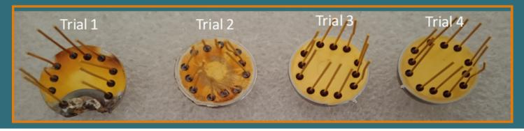
The accompanying figures illustrate an example of EBW welding between Kovar (Header) and steel (Cover), demonstrating its versatility in handling different material combinations. Multiple tests have been carried out to optimise the weld parameters, as presented in the included table.
