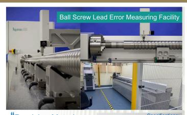
"Precision Metrology has extended its capabilities to measure Ball Screw as per ISO 3408'
