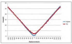
LVDT Prototype Developed by CMTI and Comparison of Voltage Vs Displacement Graph of the Developed and Commercially Available LVDT Sensor
