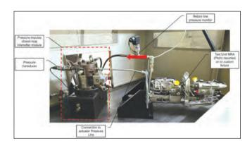
Qualification testing of Main rotor and tail rotor actuators entails testing of indigenous MR and TR actuators as per the approved Type Test Schedule (TTS). The primary rotor actuator was tested for 10,00,000 cycles of pressure impulse testing as per SAE ARP1383 A.
