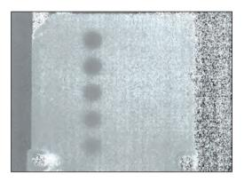
Active thermography setup for sub-surface defect detection and processed thermal image of the Aluminium sample with the circular artificial defect
