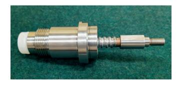
CMTI developed process technology for the machining of a 12 mm diameter, 5 mm pitch PS1 injection valve ball screw assembly. This assembly consists of ball screws, a ball nut, a sleeve, and a deflector, all featuring critical components with high dimensional and geometric tolerances ranging from 3 to 10 microns. The work was completed for LPSC ISRO Valiamala, and successfully delivered 156 sets during 2024-25.
