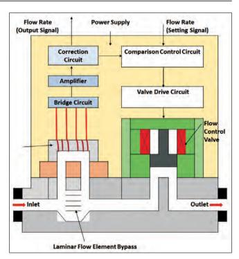
element, and the control valve, will be designed and developed with an in-house micro-machining facility. All components will be individually tested and assembled together. The initial testing of the complete MFC will be carried out at CMTI with the help of the standard MFC.
