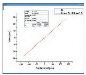
Linearity Graph between voltage and displacement for MHR 005 (commercially available LVDT)
