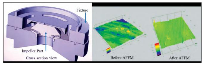
Improvement of surface roughness Ra from 14.5 µm to 3.2 µm
