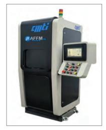
surface. As the medium flows, it forms a self-shaping mass that adapts to the contours of the workpiece, allowing for a nano-level finish on intricate micro components.
