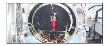
As part of the qualification testing for the modular water mist fire extinguisher, environmental tests were conducted on the test unit. These tests included humidity, sine and random vibration tests, acceleration, mechanical shock, and thermo-vacuum cycling tests. The completed unit was then handed over to M/s Ceasefire.
