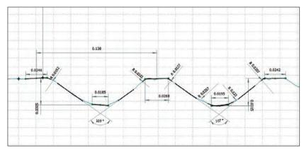
Measurement of internal micro grooves manufactured by CMTI
