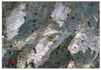
Microstructure of the printed test coupon
