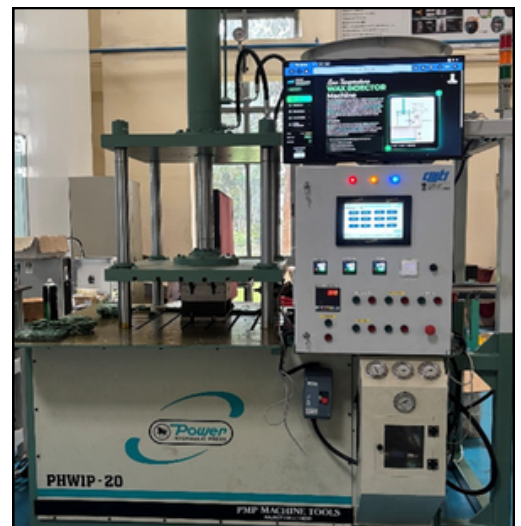
SMART LOW-TEMPERATURE WAX INJECTION MACHINE DEVELOPED
